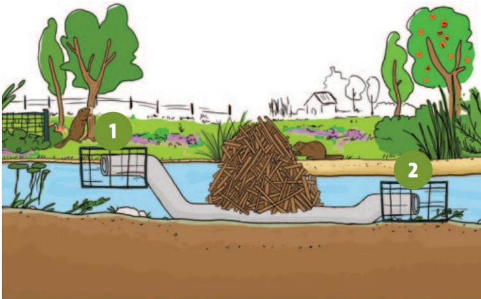
Figuur 56: Principeschets beaver-deceiver (bron: Aquafin NV)
