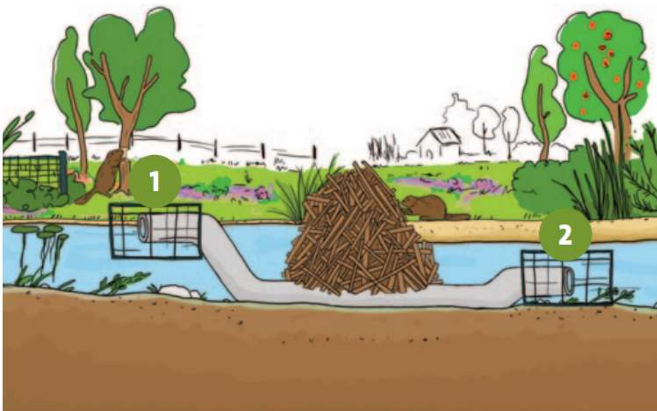
Figuur 58: Principeschets beaver-deceiver (bron: Aquafin NV)
